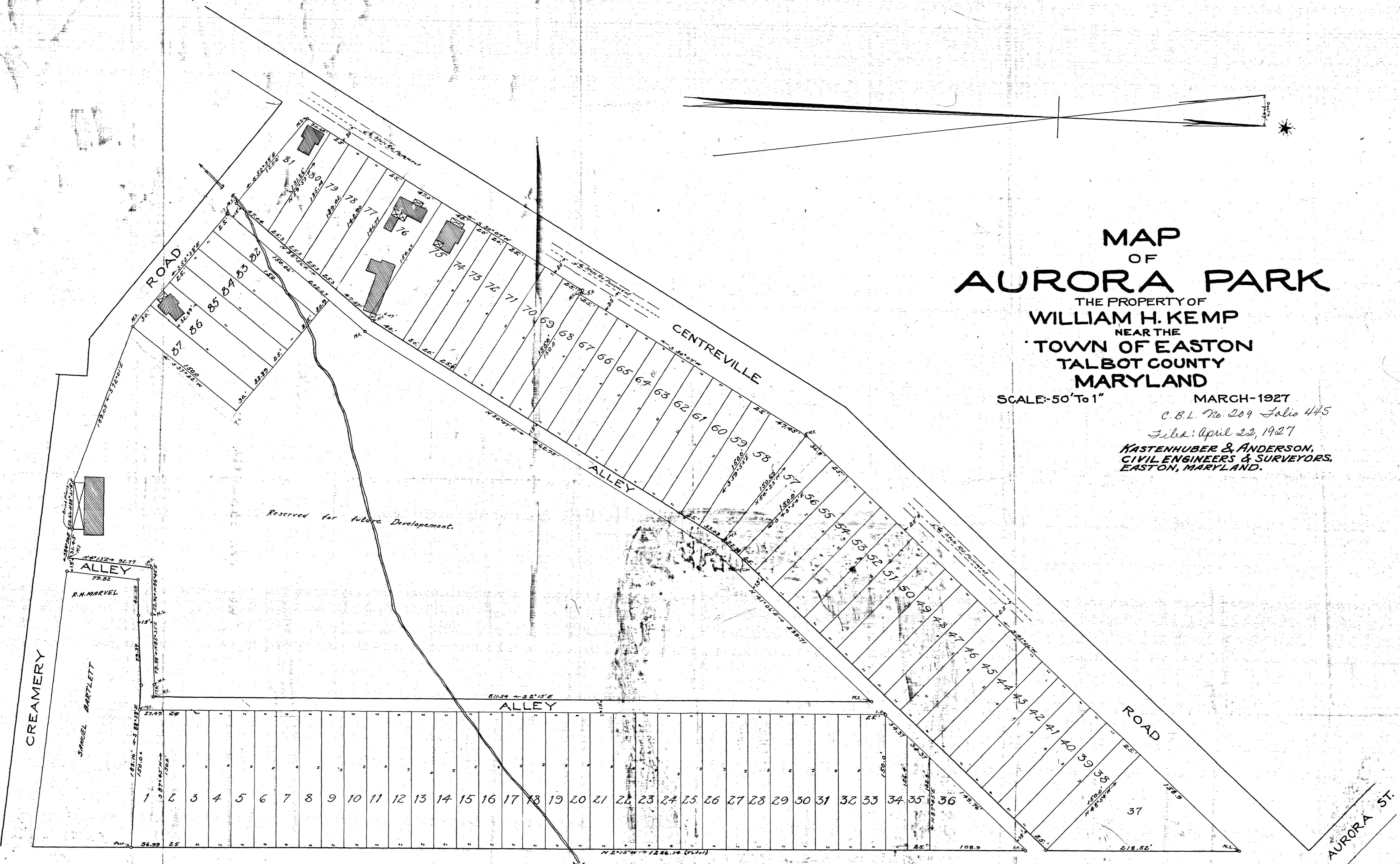
(NOTE: Bearings are computed from the angles which have been observed precisely, and are referred to a magnetic meridian corrected for the declination indicated at present being approximately..... $7^{\circ} 47'$  minutes West.)
